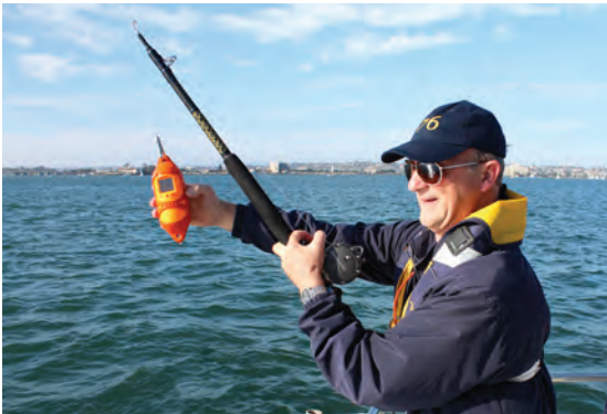
Seamless integration with the CastAway-CTD, allows sound speed corrections to be done right in the field.
