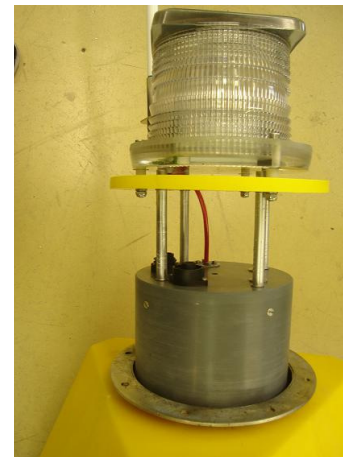
The water-tight container slides from the top into the buoy
