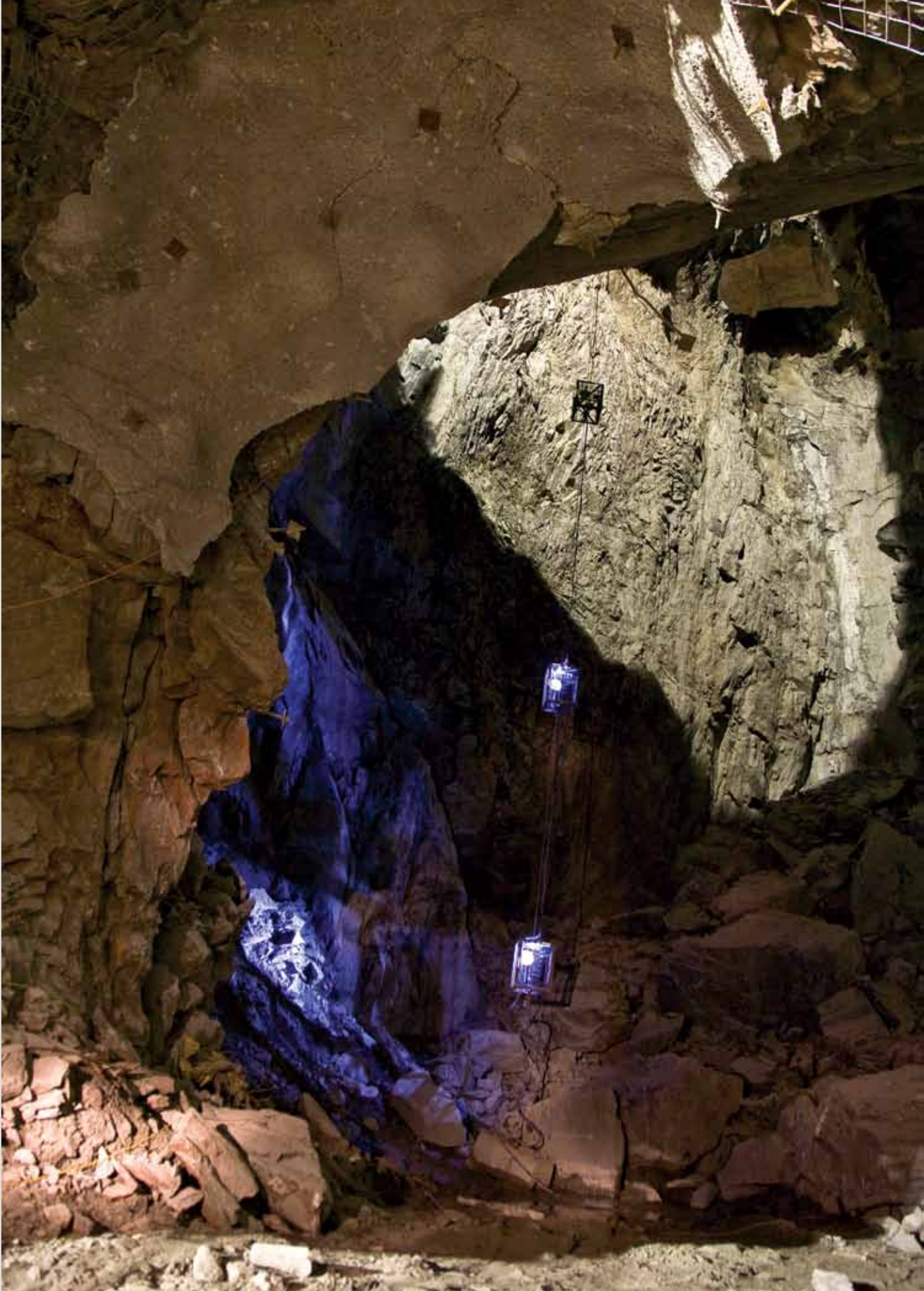
Paste Backfill Cages – Kidd Creek Mine – Timmins, Ontario Canada – Photo taken by Ryan Veenstra courtesy of University of Toronto.
