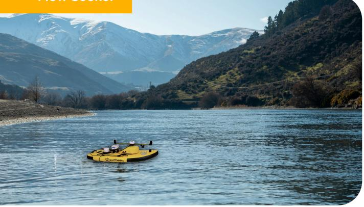
The daily driver and workhorse of the range, designed for a wide variety of gauging sections and sensor deployments. It's maneuverable, portable, and can adapt to various sensors and handle tricky situations. The inflatable hull allows for easy transportation, storage, and replacement. Autonomous transects and bathymetry as standard.
