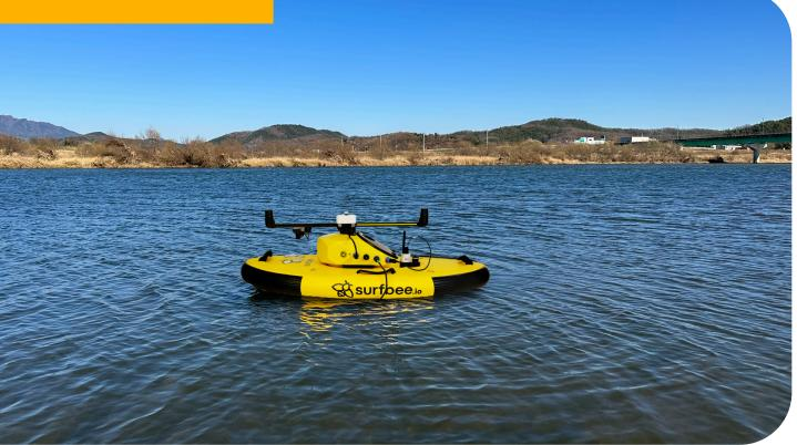
This vessel is designed specifically for Sontek RS5 deployment, taking advantage of the ADCP's new small form factor and depth range. It offers superior shallow water performance, propelled by three underwater thrusters, and features autonomous lateral movement for unparalleled vessel control in difficult conditions, such as windy, slowmoving irrigation channels.
