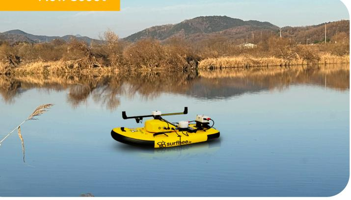
Designed for versatility, this vessel excels in shallow waters, equipped with three underwater thrusters for robust propulsion. It easily adapts to different sensors, ensuring precise control through autonomous lateral movements, even in challenging conditions like windy and slow-moving channels.
