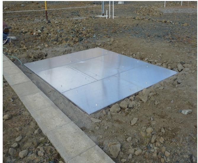
Figure 5: SGG snow scale set up Davos
