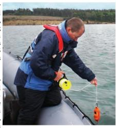
The CastAway is a multi-functional tool that incorporates the most modern technology available - yet is simple to use. It is designed for CTD profiling down to 100 m and is easy to deploy.
