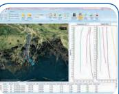
A screen capture of data from a river delta in Louisiana acquired using a CastAway-CTD. The technicians collected 21 casts in less than 3.5 hours.
