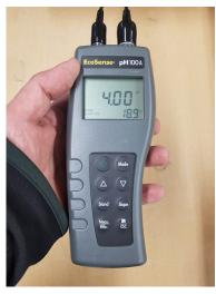
Parameters: pH Temperature mV/ORP/Redox (oxidation reduction potential)
