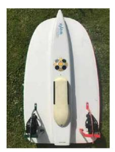
SonTek M9-Hydrosurveyor **Bathymetry and Currents** Stealth Scan Sidescan (PN SScan)
