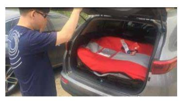
The board is able to fit in the boot of any standard sized car and weighs 8Kg. The board carry bag includes integrated shoulder straps. The controller, thrusters and power supply fit in a waterproof case with integrated wheels, dimensions D280mm by H560mm by W400mm, weight 16Kg.
