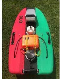
PC & Powersupply (PP ModuPC) Stealth Scan Sidescan (PN SScan)
