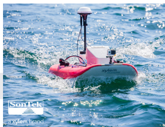
SonTek RQPod Remote Survey Boat
