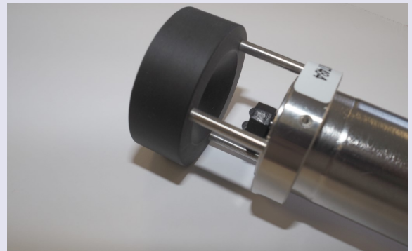
Detail of the 180° back scatter probe with deflector cone.
