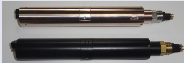
NEP5000 with wiper in copper (top) and Delrin (bottom) housing.
