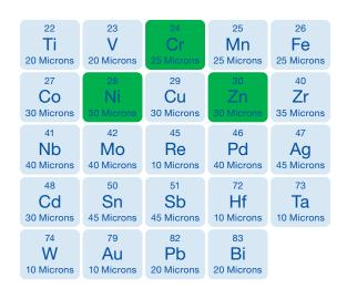
Common Elements & Maximum Coating Thickness
