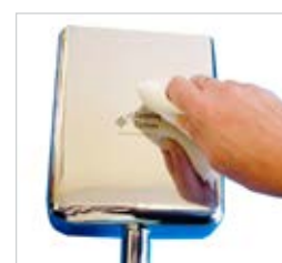
4. Clean etching area thoroughly using demineralised water
