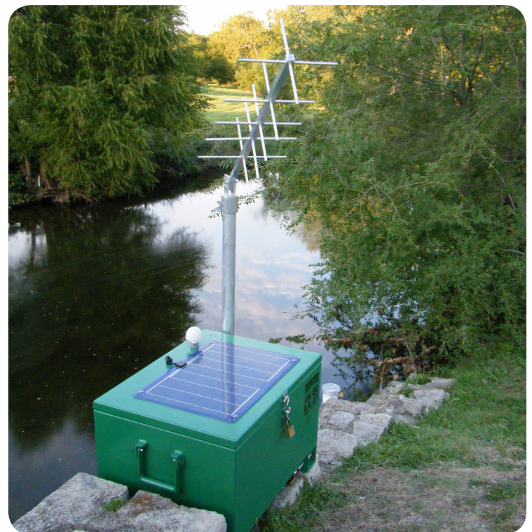
Portable aluminum chest monitoring system containing YSI Sonde and WaterLOG Data Logger. Kansas City, Kansas
