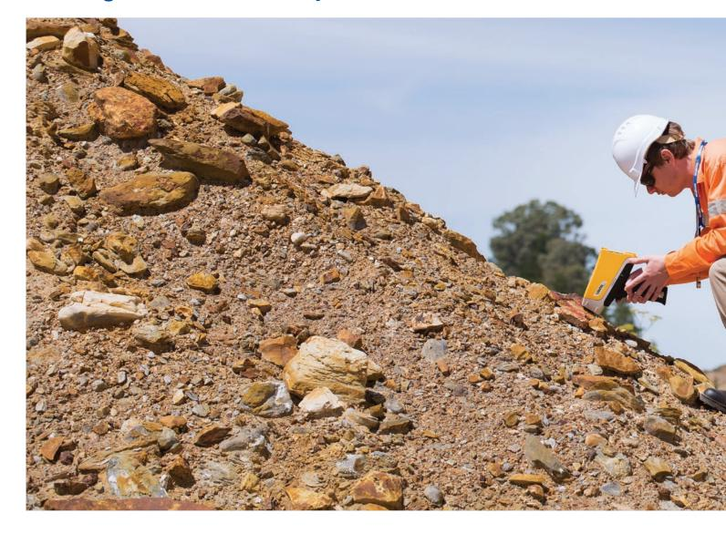
The Olympus Vanta<sup>™</sup> handheld XRF provides immediate, on-site elemental measurements for a range of geochemical applications. Vanta analyzers provide power and flexibility across the entire mineral resource cycle:
