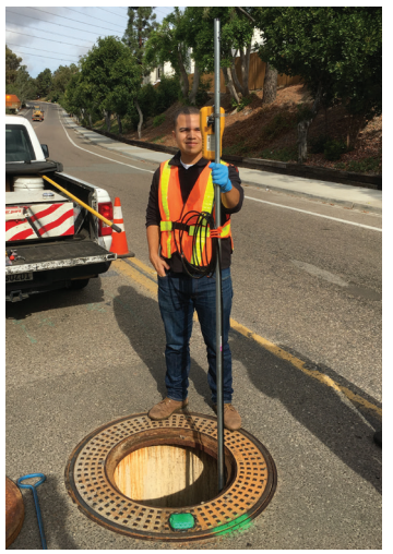
Example of FlowTracker2 used in a storm/waste water pipe.
