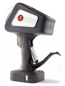
SciAps delivers portability for argon purge. With our highly efficient Optipurge™ design, a user replaceable canister in the handle delivers 500 tests. When not in use, the canister is sealed to the regulator, no gas is consumed. Don't need portability? Use our regulator attachment that mates to a larger belt-mounted argon canister or a standard stationary tank typical of spark OES analyzers.
