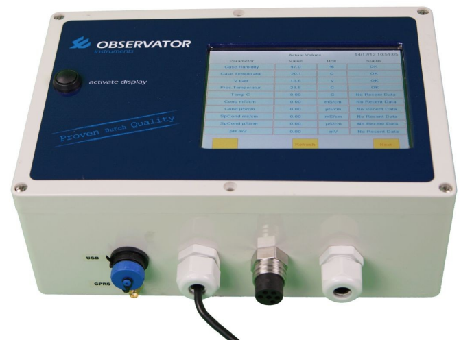
The OMC-045-III with housing and touch screen display
