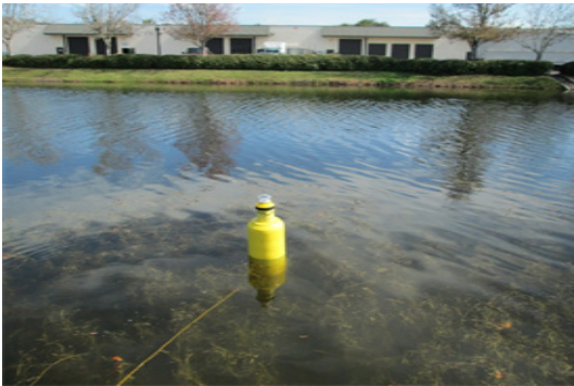
"EMM25 Buoy deployed in retention pond measuring DO"
