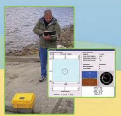
When EcoMapper is on the surface and within Wi-Fi range, view data and monitor progress. Or take manual control over vehicle.
