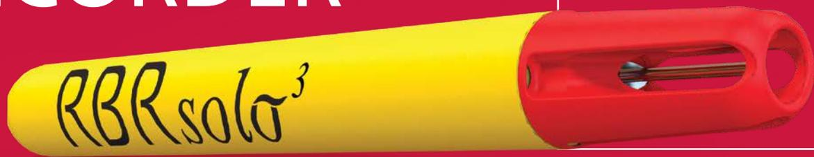
The RBRsolo<sup>3</sup> T is one of RBR's most compact, lightweight, and versatile single channel recorders. The logger offers flexible measurement schedules, standard sampling up to 2Hz (optionally up to 32Hz), large memory, extra power for extended deployments, USB-C download for large data files, and temperature accuracy of  $\pm 0.002^{\circ}\text{C}$ .
