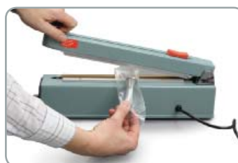
Seal the open end of the bag
