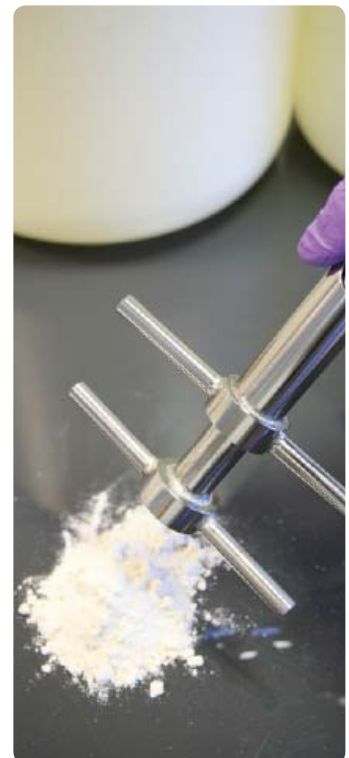
Sample being discharged from a Standard Slot Sampler without a Bottle Holder
