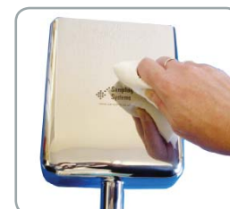
4. Clean etching area thoroughly using demineralised water
