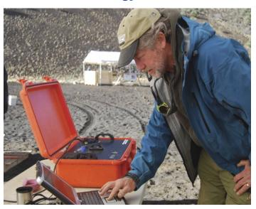
Initially conceived to perform chemical and mineralogical testing for NASA's Mars Science Laboratory (MSL) mission, Olympus' Terra™ is a rugged, fully portable field instrument which harnesses advanced dual XRD/XRF technology and renders it for earthbound applications. Combining both Olympus and NASA innovation, Terra brings to life a new way of performing X-ray diffraction and X-ray fluorescence measurements.
