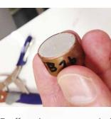
Z offers the same quantitative testing on a more comprehensive element suite with the GeoChem App. Analysis can be carried out directly on a smooth rock surface. Ideally pulverized samples are pressed and tested, typically requiring the same amount of time as HHXRF. Pressed samples can be stored in their consumable holders for later analysis or laboratory confirmation.
