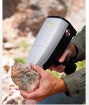
**1** - The Z LIBZ analyzer allows **2** - Users can view the sample precise targeting of specific regions on a geological sample. Simply place the Z onto the rock or core. Samples can be safely held Z is laser based.
