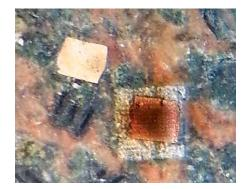
A compelling benefit of the SciAps LIBZ technology is the possibility of performing both micro analysis and bulk sample analysis. In the example below, pyritic rocks from a gold bearing ore-body are analyzed using the Z. From the user's perspective, the heterogeneous rock is viewed through the Z's high resolution camera. The laser is directed onto a region of interest, and analyzed in a few seconds. From the list elements and abundances displayed on
