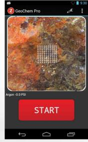
image via the on-board camera, and align the rock and adjust the raster (if needed) to strike specific zones within the sample. in the operator's hand because the Operators also view the laser during testing, and may observe the plasmas being generated. Complete spectral data is collected and analyzed at each point.
