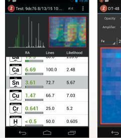
board data base of emission lines and relative intensities for every element in the Periodic Table. Elements detected are instantly presented, including qualitative relative abundances. Tap on an element, and the spectral view zooms to the relevant spectral lines. A "thumbnail" shows the heat map for that element, by position in the sample
