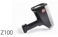
Smaller and lighter hand held LIBZ analyser. Great alternative for many HHXRF applications. Enables analysis of elements as light as Li [Z=3], as heavy as U [Z-92] - does not have argon purge, will not analyse Carbon [C]. Provides excellent detection limits, incorporates a high powered pulsed laser, a mid range resolution spectrometer [200-850nm] and medium sized display.
