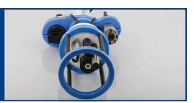
The RBR*maestro* can be equipped with any 13 channel combinations.
